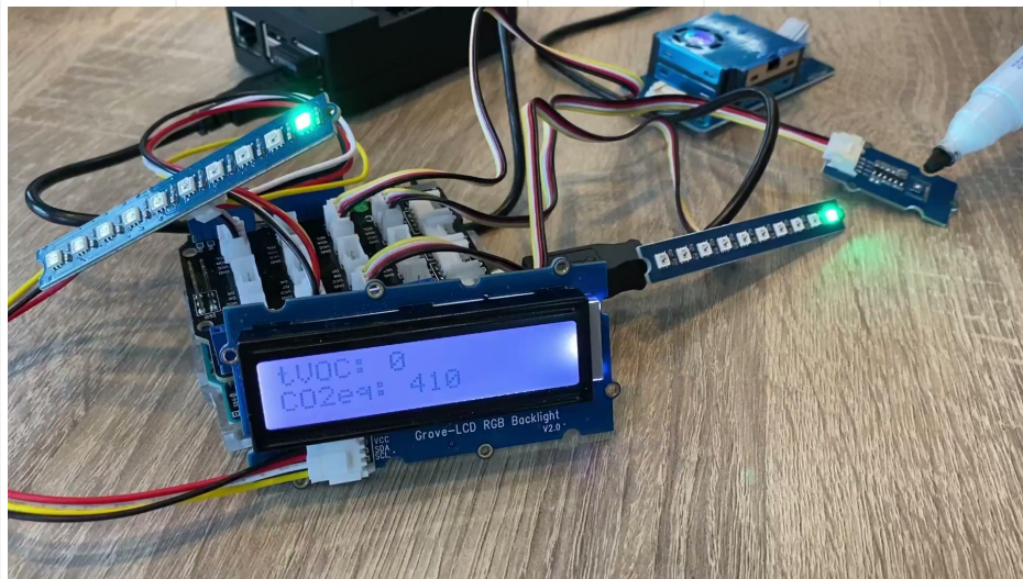
Gas sensor reaction, readings, LCD display and averaged reading
